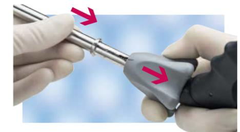
**III** Pull star wheel back and insert shaft. Marking on star wheel and marking on shaft should line up.
