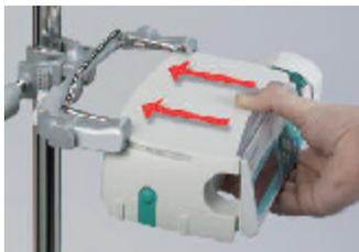
Space Pole Clamp will rotate 360° and lock into place in 45° angles, allowing you to clamp to horizontal or vertical poles
