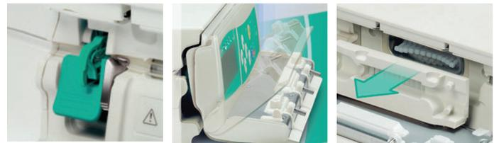
Anti-free flow clamp built into set and pump and removal mechanism
